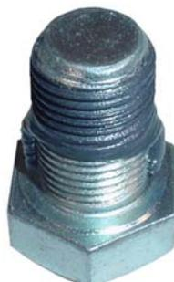
The same bolt is also shown after a nut was partially assembled and then removed. The two beads of compound have been dispersed into the threads by the rotation of the nut. Although not shown, the leading edge of the nut was almost clean indicating that most of the compound was dispersed into the threads by the rotation of the nut.
