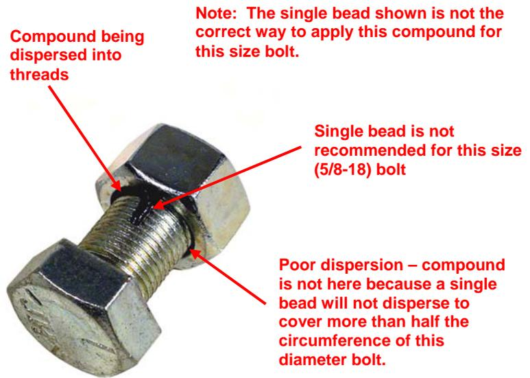
The **bead diameter** is calculated to obtain a 0.3 mm thickness (0.012”) on the surface area of the male threads. Larger than specified bead diameters may allow some compound to build up on surface of the nut instead of allowing it to be dispersed into the threads.
