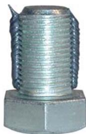
Automatic application of anti-seize compound uses a robot to move the bolt past a stationary nozzle while the compound is extruded. The bolt shown has 5/8-18 threads 1" long. Compound was applied as two 0.140" diameter beads for a total volume of 0.51 cc (0.255 cc per side).
