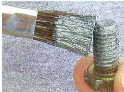
Photo shows typical manual application of an unknown quantity of anti-seize compound using a brush. This is not practical in an automatic assembly cell.
