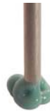
Grease may not stick to part because nozzle is too far from part
