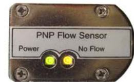
LED's showing Power and No Flow
